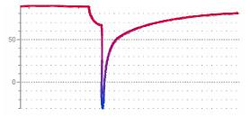
RAM blasted with Difluoroethane (aerosol propellant).
