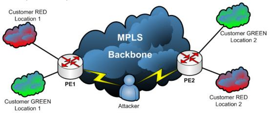
The attacker is in a Man-in-the-Middle situation inside the data path between Provider Edge 1 and Provider Edge 2 in the MPLS backbone.
