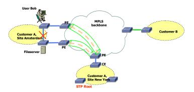
Here the network traffic resulting from Bob's access to the fileserver with actually be forwarded to New York and back to Amsterdam (as the link between the switches in Amsterdam is in *blocking* state), effectively passing the MPLS backbone (possibly unencrypted). Moreover Bob (or the site's or the company's security officer) might be completely unaware of this situation.
