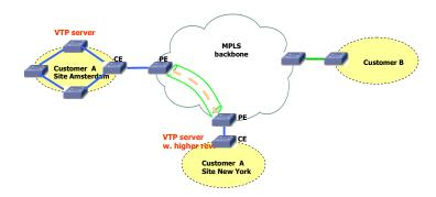
With a fully transparent Intra-Site Ethernet connection the switch in New York will propagate it's VLAN table to the switches in Amsterdam effectively melting down the complete network over there<sup>10</sup>.
